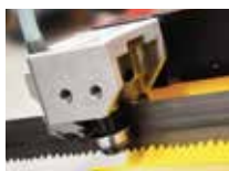
Saw blade guide made from carbide
